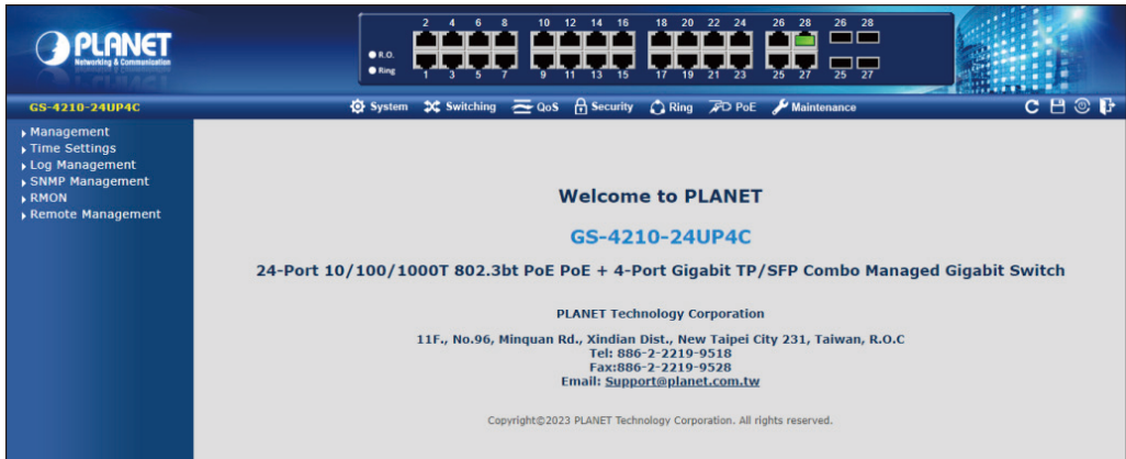
Figure 4-6: Web Main Screen of Managed Switch
